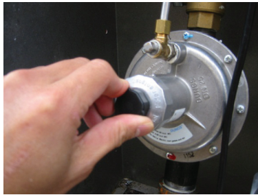
Figure 6A - Dungs FRG Ratio Regulator Adjustment - Figure 6B
