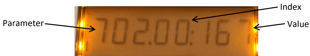
Figure 7-1: LME7 Fault History Example with Indexes
