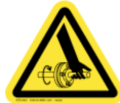
Entanglement of Hand/Rotating Shaft
