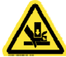
Hand Crush from above
